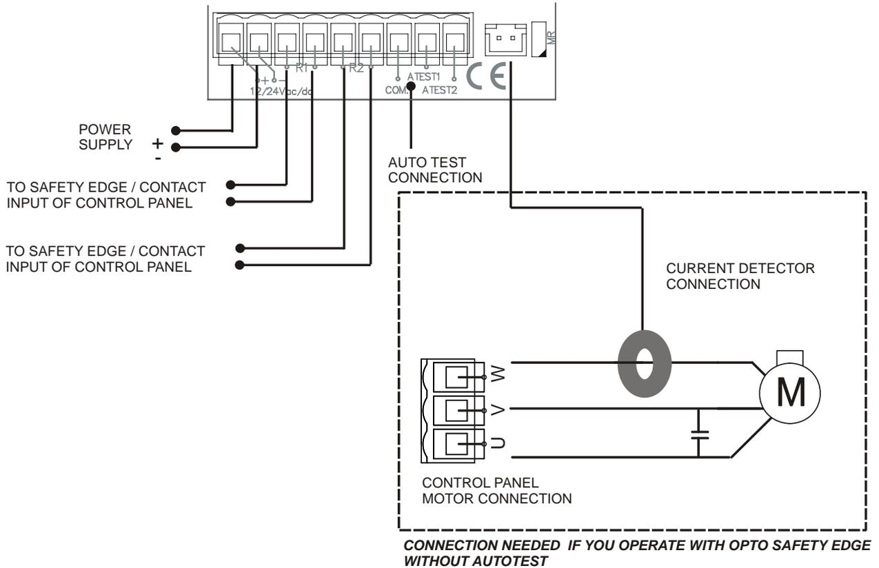
The outputs can be configured to act an 8k2 or as a N/C Contact.
