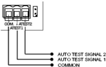
THE RADIOBAND RECEIVER WILL ACCEPT TWO TYPES OF AUTO TEST SIGNAL. THE FUNCTION SELECTOR SWITCH MUST BE PUT IN THE CORRECT POSITION FOR THE AUTO TEST SIGNAL.
