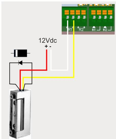
**AC inductive loads:** 30Va / 30Vac / 1A -> 750000 manoeuvres. A varistor (V68ZA2) with electric lock or suction cups is necessary in parallel.
