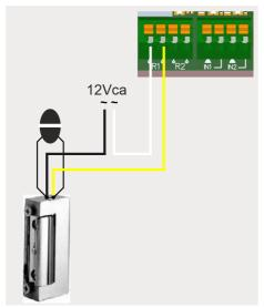
If using suction cups, the relay type must be "Normally closed" (see: "Configuring relays and assigning traffic schedules").
