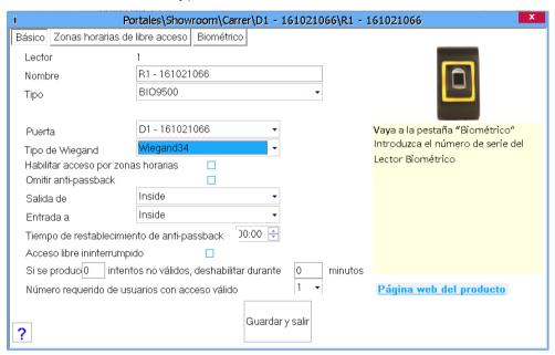
4. After selecting the type, a third tab will appear "Biometric". Go to that tab and put the serial number of the Biometric Reader.
