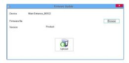
The default location of the firmware files installed with CONTROL is in the folder "Firmware". Select the firmware file with a "xhc" extension. Click on the Upload button.
