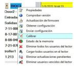
**Note:** It is recommended to do a calibration while commissioning the reader and in cases when there are problems with reading the fingers.
