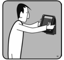
HANG CONTROL PANEL
