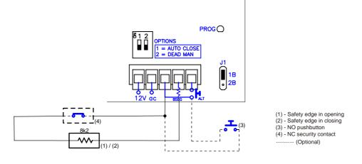
A security device (photocells, normally closed contact) can be connected in series with the safety edge. The activation of this security device causes a stoppage and a total reversion of the door.
