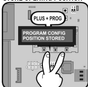
PRESS PLUS + PROG TO STORE OPENING POSITION
