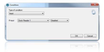
For an "External input" condition, select the input to be tested (only those in IP-EXTIO modules) and then select its status (enabled, disabled or sabotaged for the four-state inputs of the IP-EXTIO modules).
