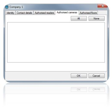
From this tab, you can select which cameras will be used by the company. This means that the company can only display and/or drive these authorised cameras.
