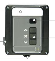
With Display card, viewing of operating status and parameter configuration
