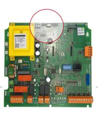
Although the board already includes 27 radio codes as standard, we also give you the option of expanding the number of codes to 500 users... using the MEM500 memory card. You can manage installations with the Soft-Assistant programming tool.
