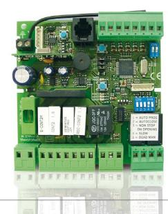
DC operating panel for swing, sliding, up-and-over and sectional doors.
