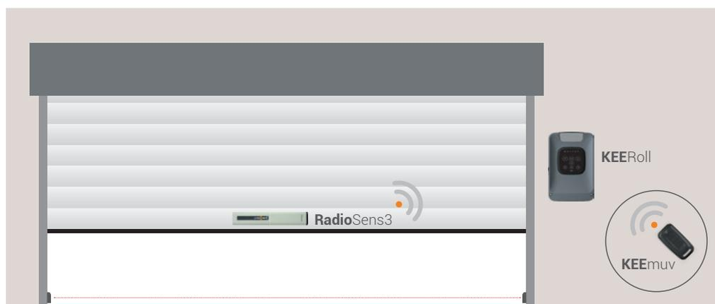
KEERoll application in roller shutter with RSens3 system (without safety edge).
